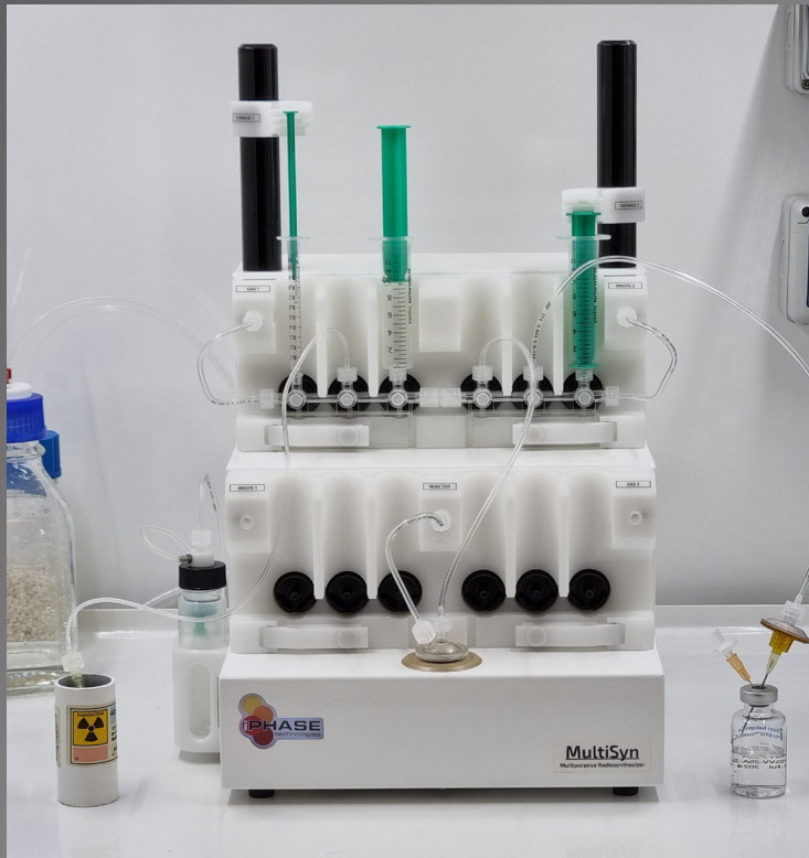
Setup for ^{177}\text{Lu} -PSMA & ^{177}\text{Lu} -DOTATATE radiolabelling.
