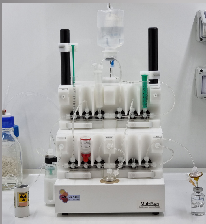
Setup for ^{89}\text{Zr} radiolabelling.
